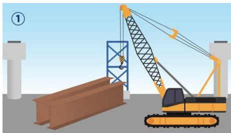
1. A large crane lifts the steel girder.
