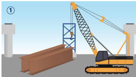
1. A large crane lifts the steel girder.
