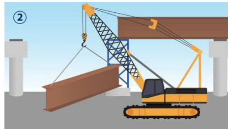
2. The girder is lifted in place to connect the bridge piers. A temporary tower supports the girders as they are safely secured.
