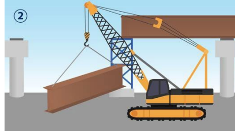
2. The girder is lifted in place to connect the bridge piers. A temporary tower supports the girders as they are safely secured.
