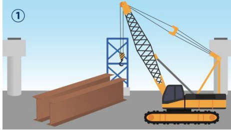
1. A large crane lifts the steel girder.
