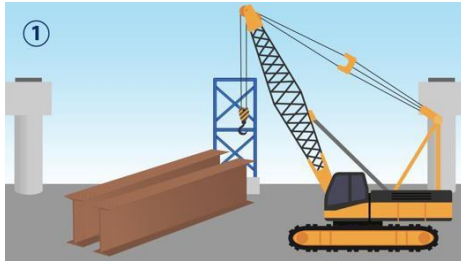
1. A large crane lifts the steel girder.
