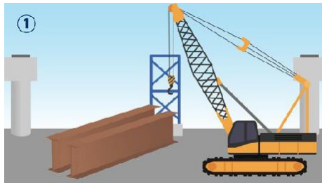
1. A large crane lifts the steel girder.
